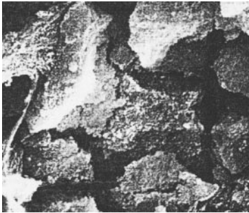
Figure 7.31. Particle splitting. [Adapted, by permission, from Li J X, Silverstein M, Hiltner A, Baer E, J. Appl. Polym. Sci. , 52 , No.2, 1994, 255-67.]
