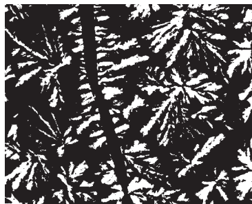
Figure 7.18. Optical micrograph with crossed polars of bamboo fiber in maleated polypropylene. [Adapted, by permission, from Mi Y, Chen X, Guo Q, J. Appl. Polym. Sci. , 64 , 1997, 1267-73.]
